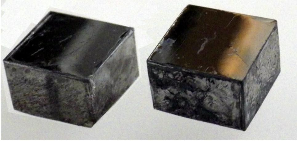
Figure 4: AluBor4 samples coated with  $m = 3$  super-mirror after irradiation. Fluence on the irradiated surface:  $7.70 \times 10^{17}$  n/cm<sup>2</sup>.
